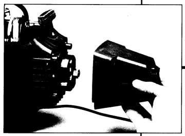
• 5. Separate clutch drum housing asssembly from engine.
