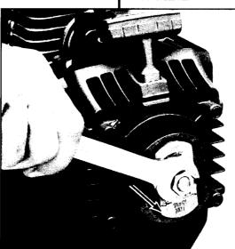
6. Remove clutch retaining nut by turning counterclockwise with a 9/16 wrench. With nut removed, clutch will slide off crankshaft with the beveled washer and large flat washer behind the clutch.
