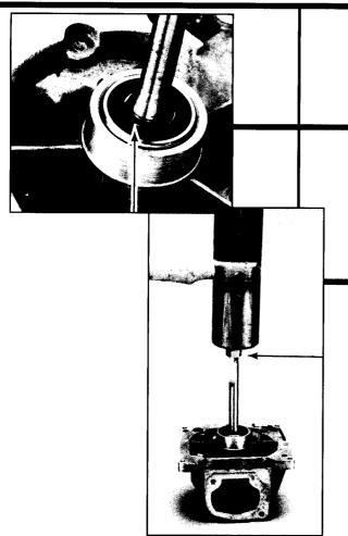
14. Remove snap ring next to bearing with snap ring pliers.
