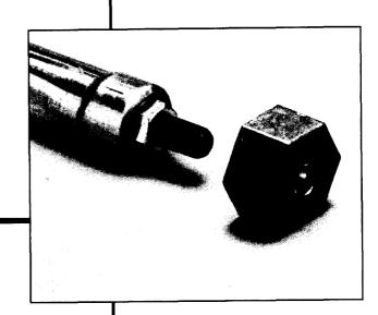
2. Once in place hold dust cap with a wrench to prevent arbor shaft from turning on 26 RLC and 26 LC units. On straight shaft units use the locking pin to hold dust cap from turning.
