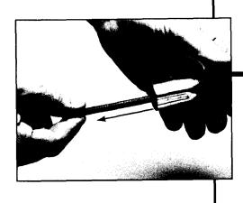
4. Remove drive shaft from drive shaft housing.
