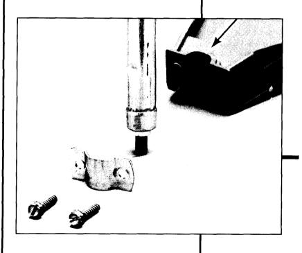
1. Match the key (raised area) on the shield with "V" slot on drive shaft housing.
