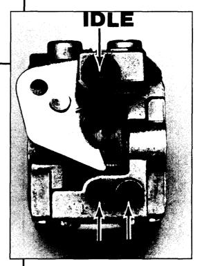
The trimmer head should not rotate after the low speed has been adjusted. If so repeat the IDLE SPEED ADJUSTMENT procedure and check LOW SPEED MIXTURE ADJUSTMENT again.
