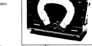
4. Squeeze the filter and allow to air dry.
