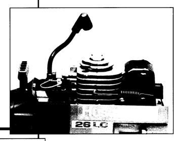
Remove throttle wire from throttle trigger assembly.
