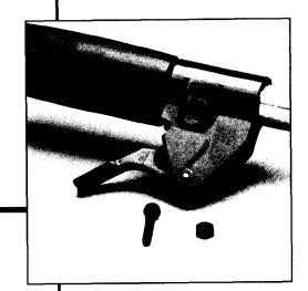
2. Carefully pull throttle trigger away from foam grip handle, then remove barrel end of throttle cable from the throttle trigger. Carefully pull throttle cable out of foam grip.
