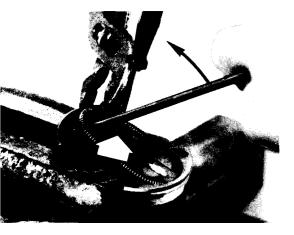
Secure the clutch hub in a vise. With the assistance of a screwdriver and a pair of pliers, lock the remaining clutch shoe so that the spring groove is exposed, then install the spring.
