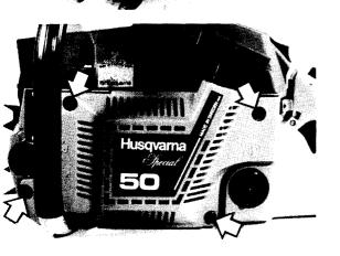
Release the grip so that the pulley engages the starter pawls on the flywheel. Install and tighten the four starter retaining screws.
